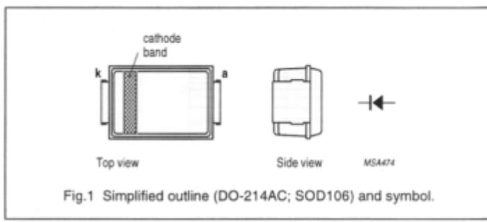
Fig.1 Simplified outline (DO-214AC; SOD106) and symbol.
