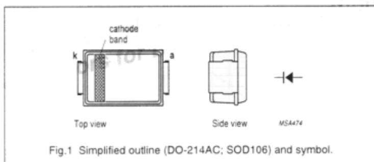
Fig.1 Simplified outline (DO-214AC; SOD106) and symbol.
